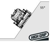
Stability and grip of the vehicle on difficult terrain up to 55° slopes under optimal conditions
